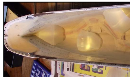
Rounded corners of plastic milk bottles were cut out as initial baffle for the LEDs, these also served to provide a platform for the horizontal sheet of opaque plastic.
